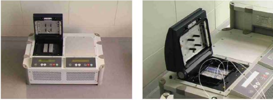
Figure 2: Clemens-Thermocycler with three temperature zones that can be cycled individually.
